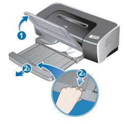
• Open the top cover. The print cartridge carriage should return to the right side of the printer. If the carriage does not return to the right side, turn off the printer, and then move the carriage to the right. Pull any jammed paper towards you.
